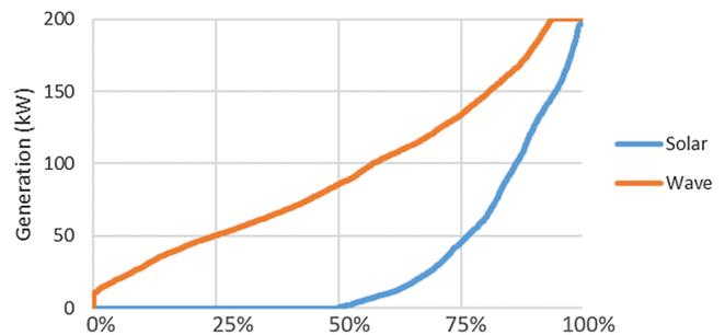
Fig. 20. Solar and wave sorted by generation output.
