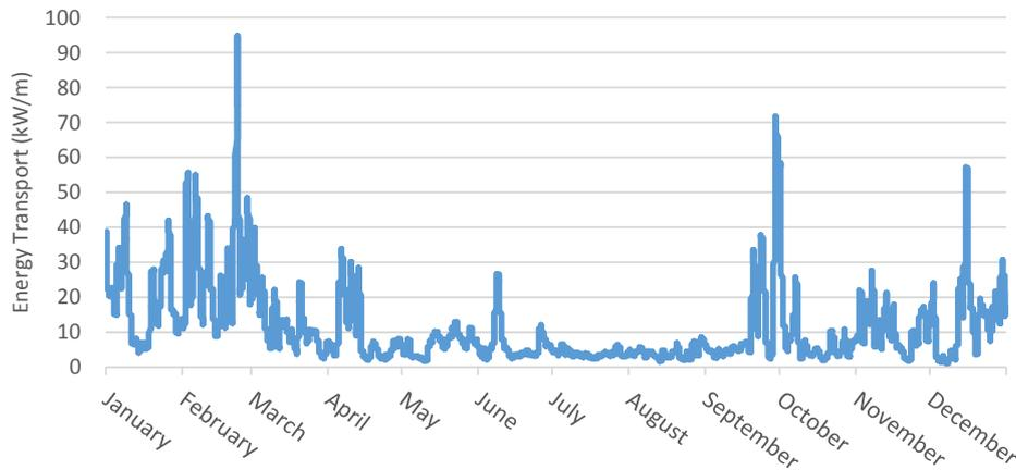
Fig. 7. Wave energy transport at Hot Springs Cove in 2013.
