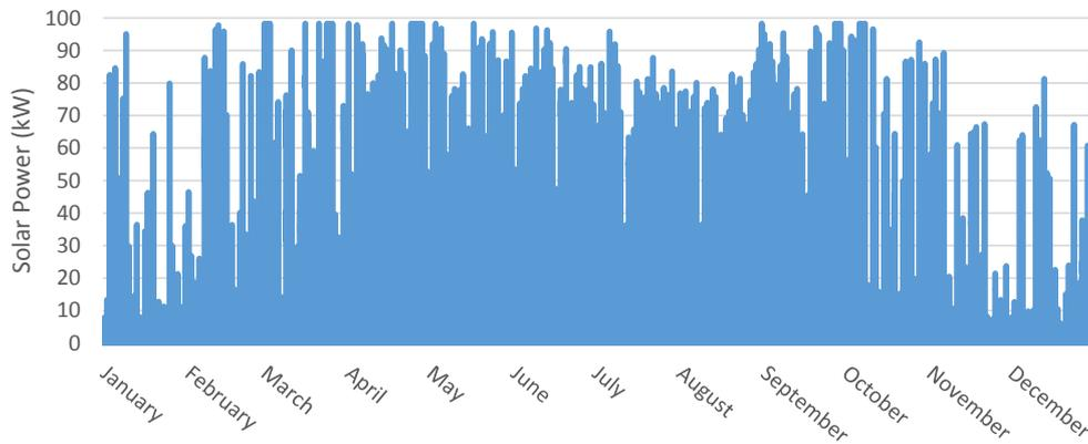
Fig. 10. Solar PV output at Hot Spring Cove.
