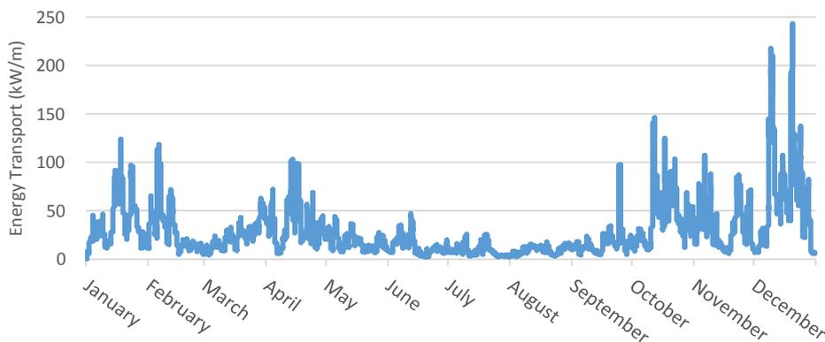
Fig. 6. Wave energy transport at Hot Springs Cove in 2015.
