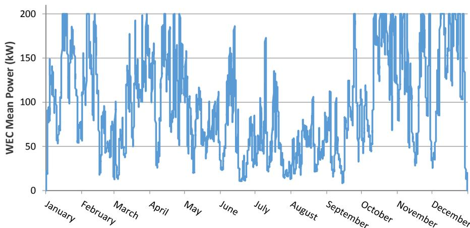
Fig. 13. 200 kW WEC power generation at Hot Spring Cove.
