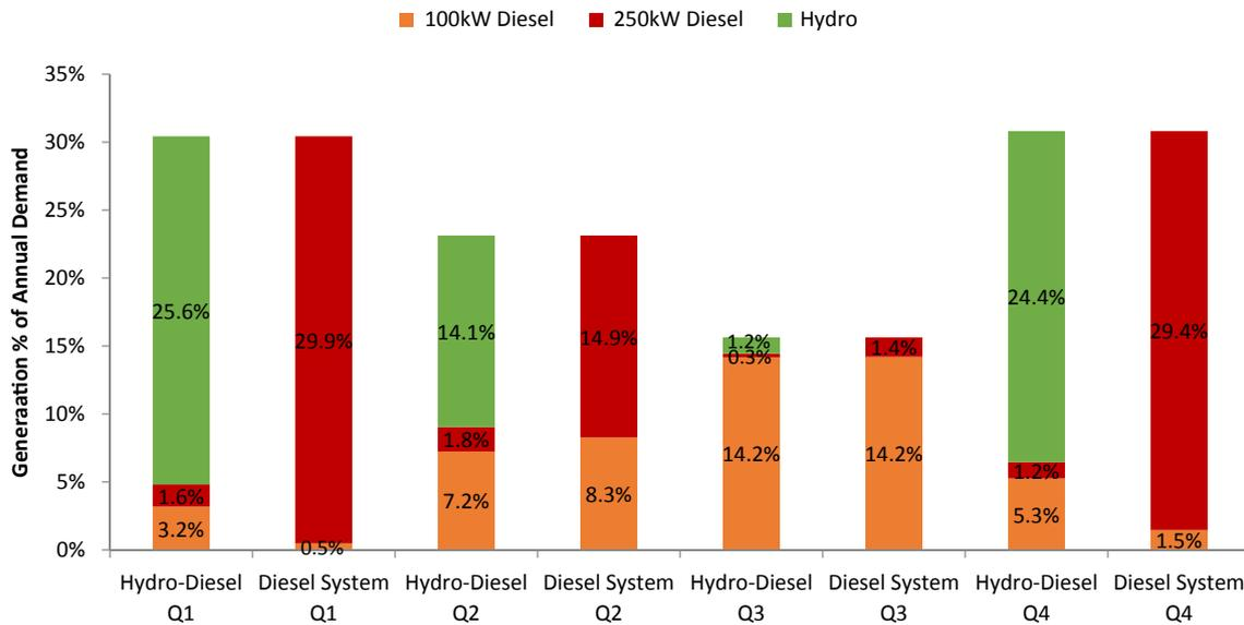
Fig. 14. Hydro-diesel system generation.
