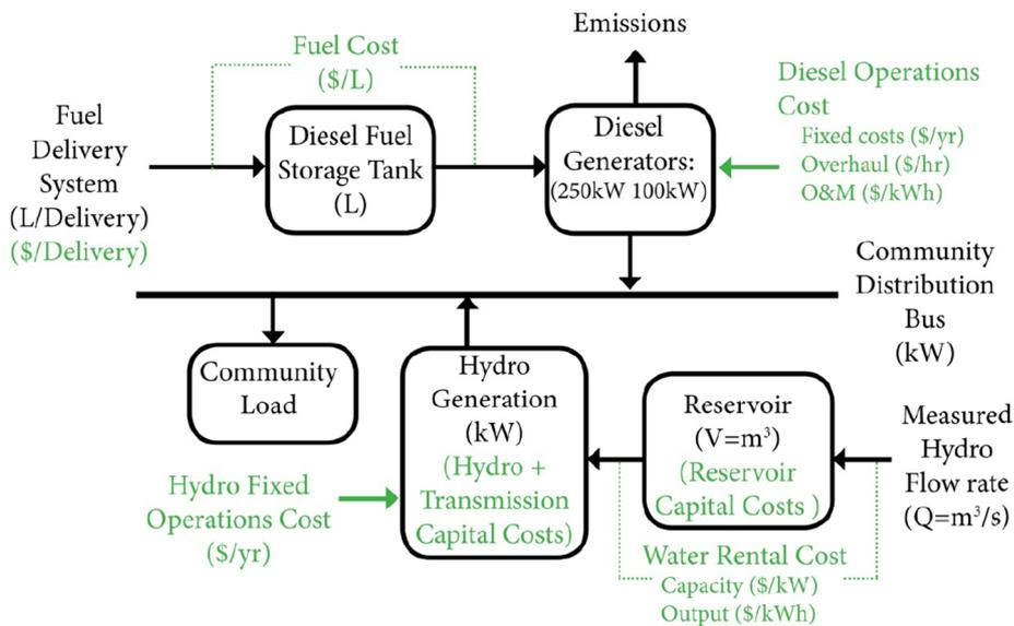
Fig. 2. RCOM economic analysis for hydro-diesel example system.
