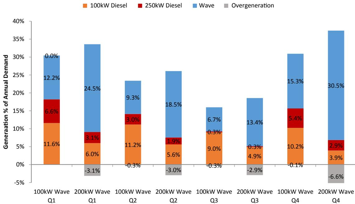
Fig. 16. Wave-diesel system generation.
