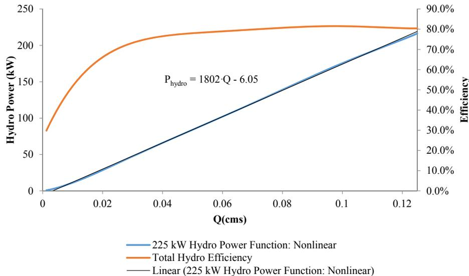
Fig. 9. 225 kW Hydro-electric generation power relationship.
