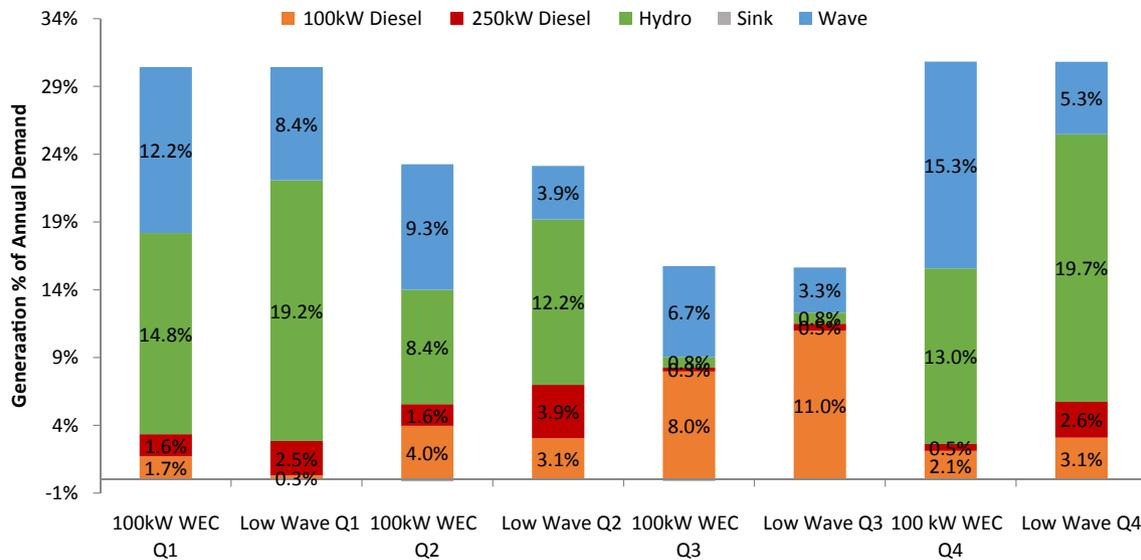
Fig. 19. Wave-hydro-diesel system generation – low and high wave scenarios.
