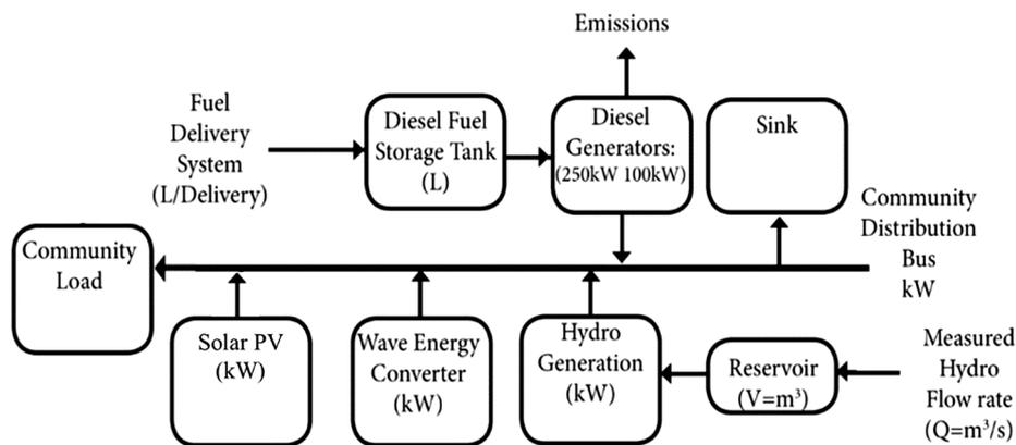
Fig. 8. Complete hybrid energy system options for Hot Springs Cove. Each energy system scenario includes/excludes certain generators from system as described in Table 3.
