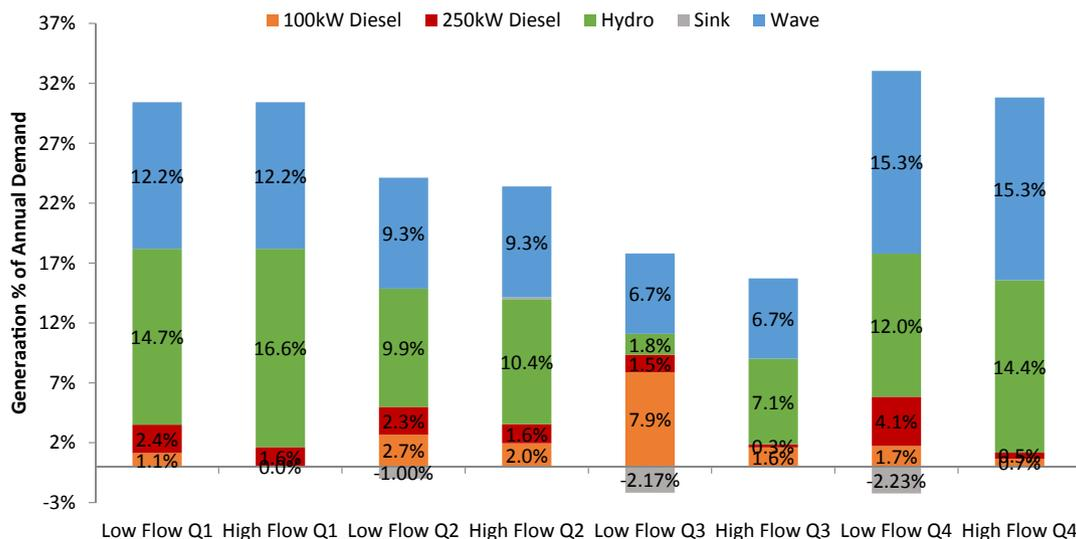
Fig. 18. Wave-hydro-diesel system generation – low and high flow scenarios.
