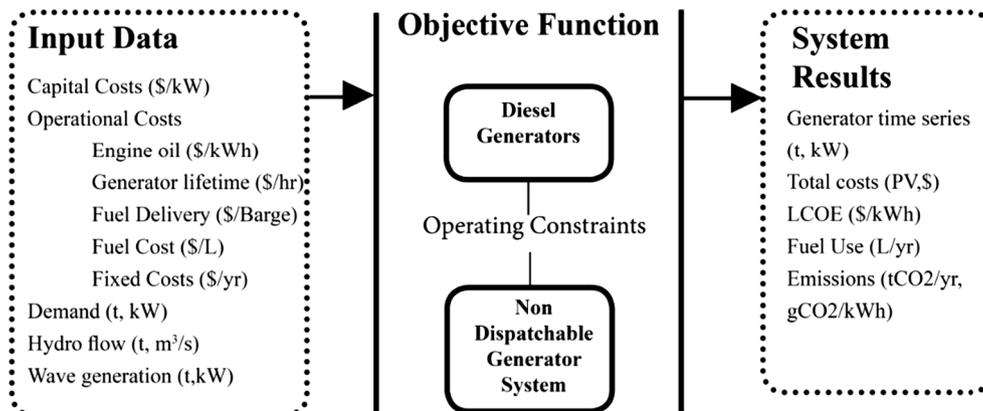
Fig. 1. RCOM process example – hybrid hydro-diesel energy system.
