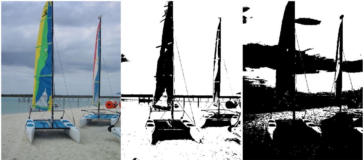
Figure 2.14 (Top) Iterative selection applied to the text and line image. (Bottom) Image of a wind surfer thresholded using iterative selection (center) and the mean value (right).
